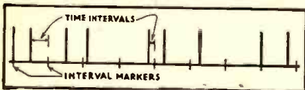
Fig. 3—PTM signals and interval markers.
